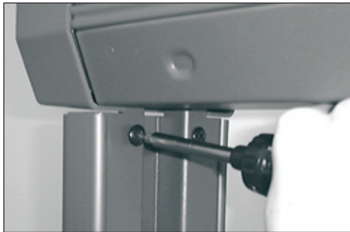
Figure 10. Insert Screws in legs or cradle feet.
