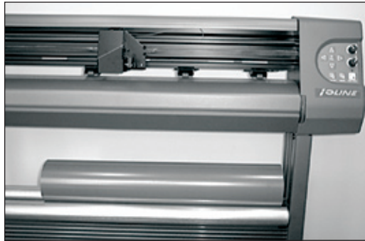
Figure 15. Vinyl loaded on media roller.
