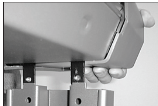
Figure 8. Place cutter on stand.
