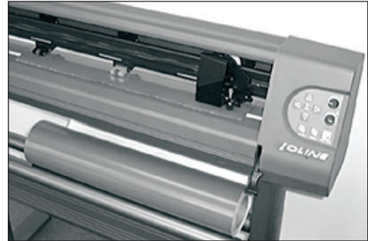
Figure 18. Leave slack in the vinyl.
