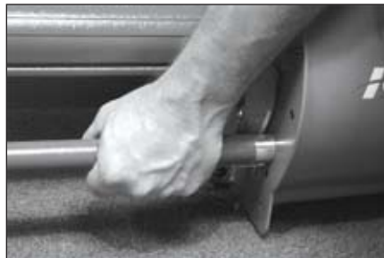
Figure 1. Lift the printer head using the gray bars to avoid injury to your fingers.
