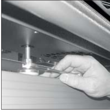
Figure 17. Leveling pads keep the platen level, helping to maintain paper alignment.
