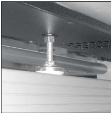
Figure 18. Tighten the jam nut against the bottom cover after you adjust the leveling pad.
