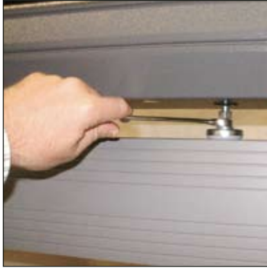
Figure 21. Leveling pads keep the platen level, helping to maintain paper alignment.
