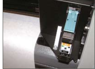
Figure 29. Do not cover the hole in the platen with paper
