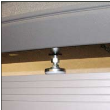
Figure 22. Tighten the jam nut against the bottom cover after you adjust the leveling pad.
