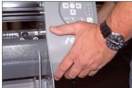
Figure 1. Hold the bottom surfaces of the end covers to avoid injury to your fingers. (See also Figure 9 .)
